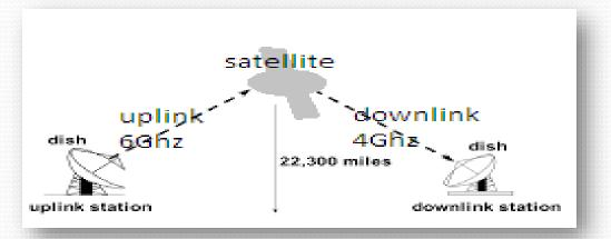
It support Very Long Range Communication with Line of Sight Propagation . It Cannot Penetrate Solid Objects. It is Very Expensive communication mode.
